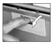
1) Remove the metal grease filters.
